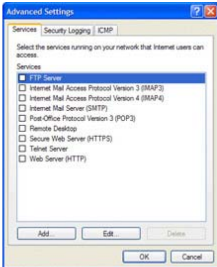
Figure 18.7 : Configuring the Internet Connection Firewall's advanced settings
