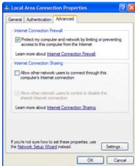
Figure 18.6 : Activating Windows XP's built-in firewall
